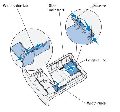
Load print media into any of the standard or optional trays. All trays are loaded the same way.
